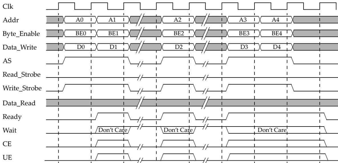
Figure 3-6: LMB Back-to-Back Write Operation
