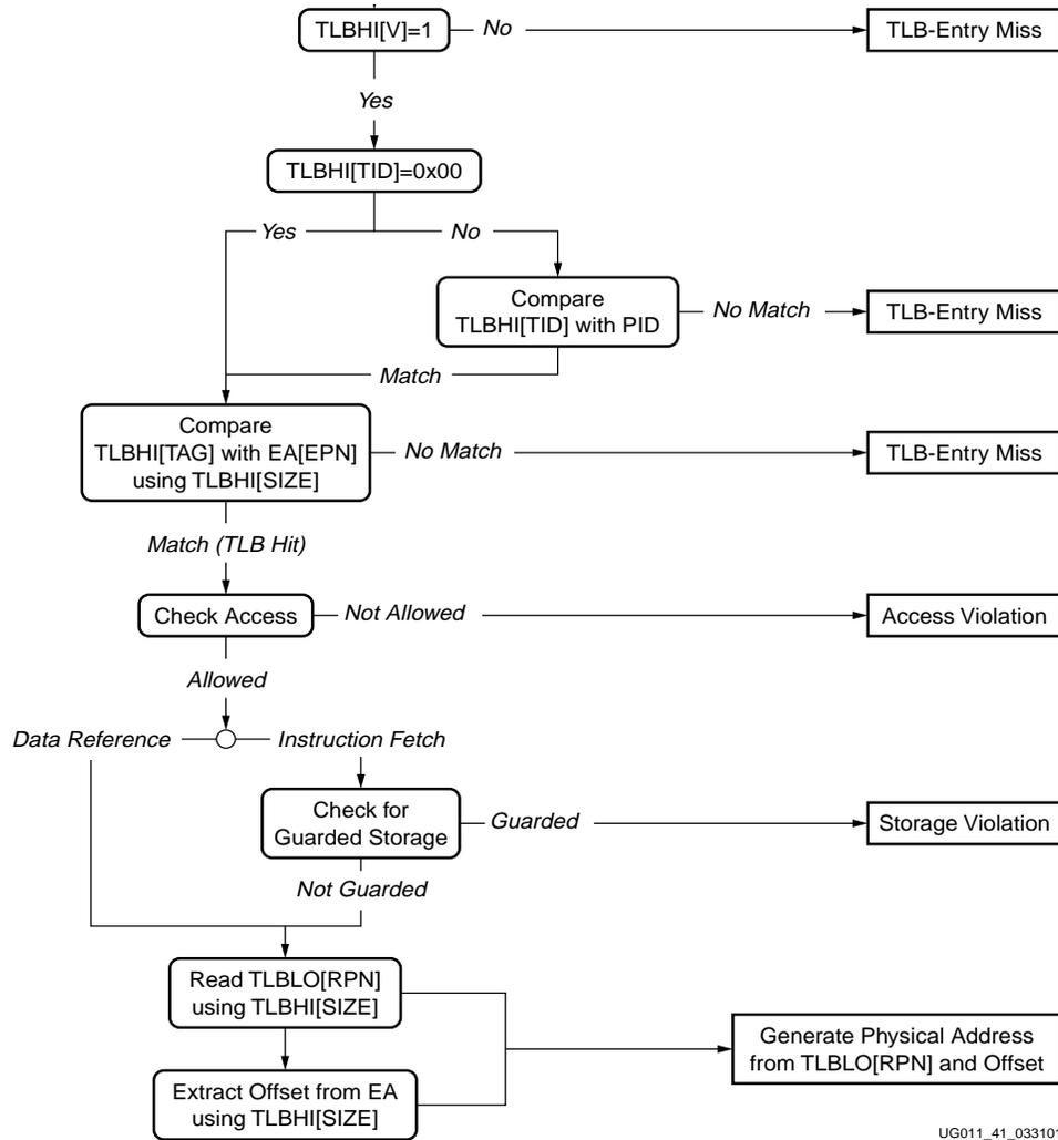
Figure 2-21: General Process for Examining a TLB Entry
