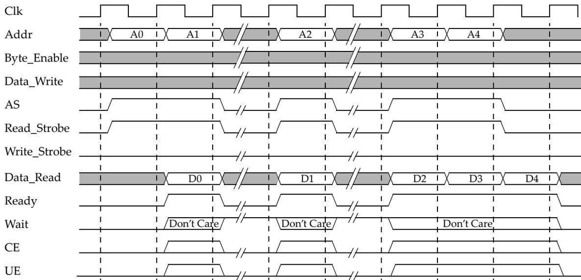
Figure 3-7: LMB Back-to-Back Read Operation
