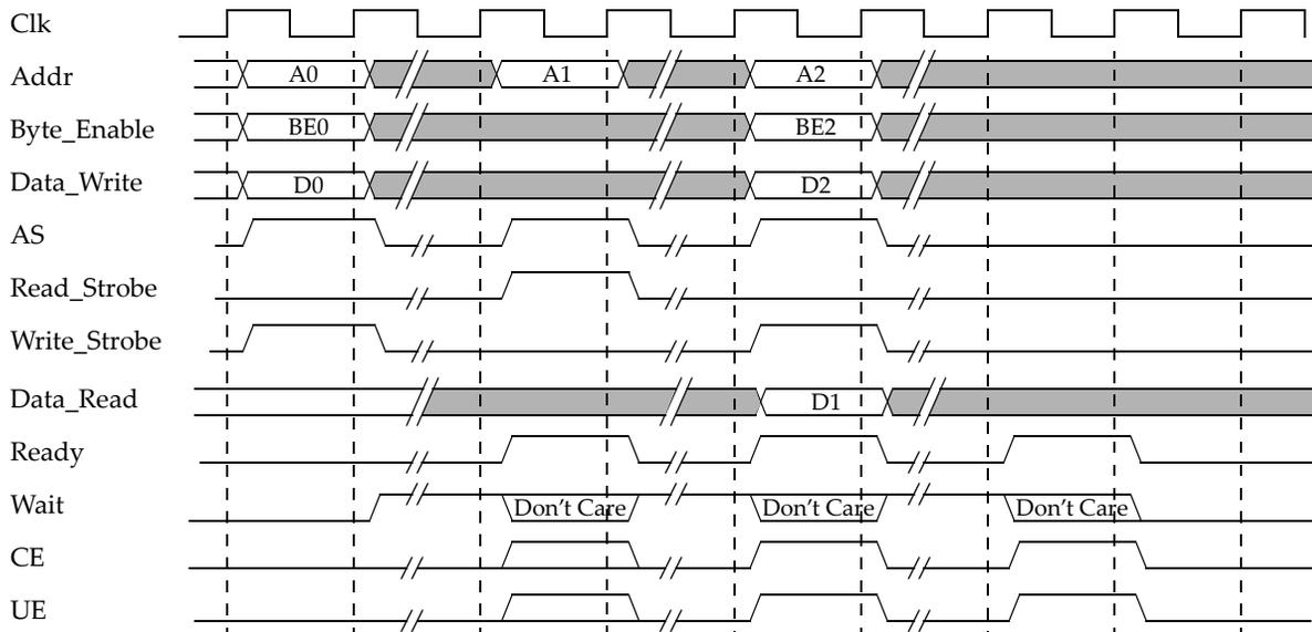
Figure 3-9: Back-to-Back Mixed Write/Read Operation, N Wait States
