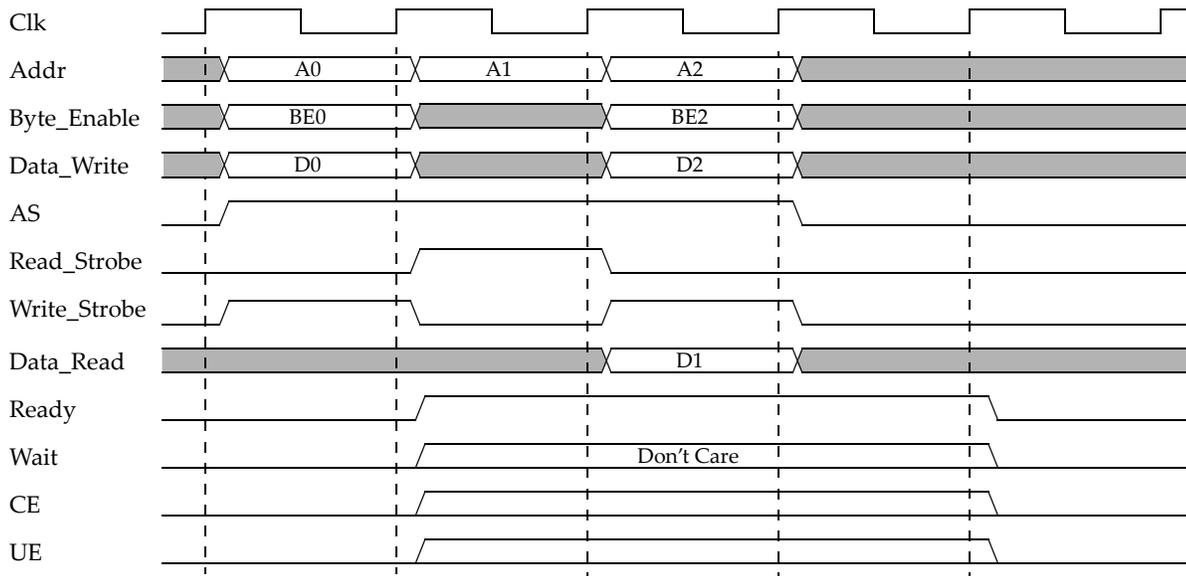
Figure 3-8: Back-to-Back Mixed Write/Read Operation, 0 Wait States
