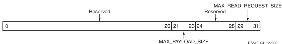
Figure 4: PCIe Request Control Register
