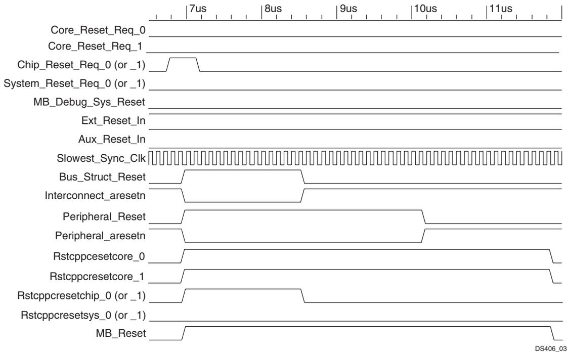
Figure 3: Processor System Reset Module - Chip\_Reset\_Req
